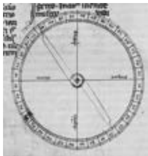
Pivoting compass needle in a fourteenth-century copy of 'Epistola de magnete' of Peter Peregrinus (1269).
